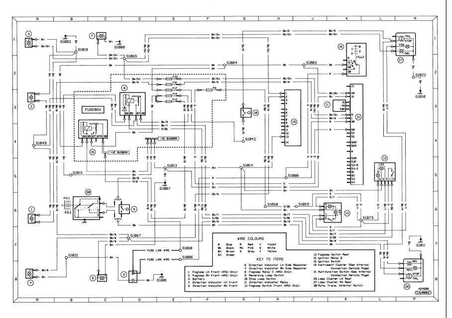
Diagram 2a: Exterior lighting - stop, reversing, fog and direction indicator lamps
